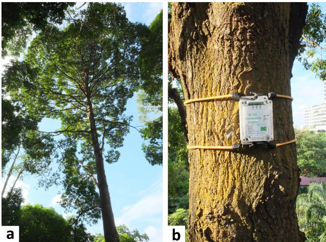
481 Figure 1 The ambient vibrations of one Hopea odorata Roxb. (Dipterocarpaceae) (a) were 482 monitored using an accelerometer attached to the trunk immediately below the crown (b).
